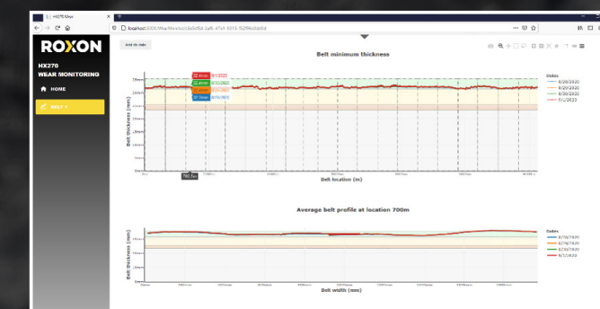
BELT MINIMUM THICKNESS AND CROSS-SECTION FROM ANY LOCATION
